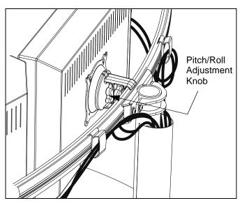
Figure 14: Display Pitch and Roll Adjustment
