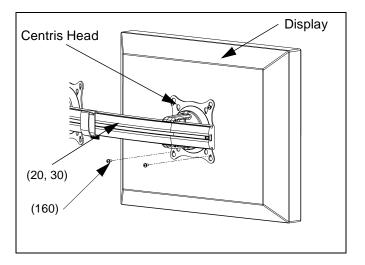
Figure 7: Secure Display to Centris Bracket
