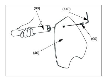
Figure 2: Assemble Pole to Base
