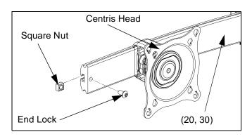
Figure 8: Remove End Lock(s)
