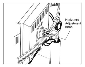
Figure 13: Display Horizontal Adjustment
