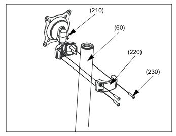
Figure 3: Mount Centris Head with Pole Clamp
