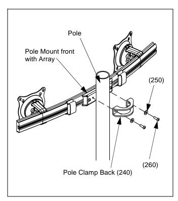
Figure 4: Assemble Array Rail to Pole
