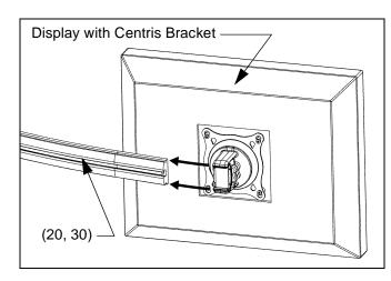
Figure 11: Mount Display with Centris Bracket to Array Rail
