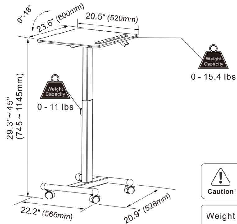
**Caution!** Do not exceed the max. loading capacity as shown.
