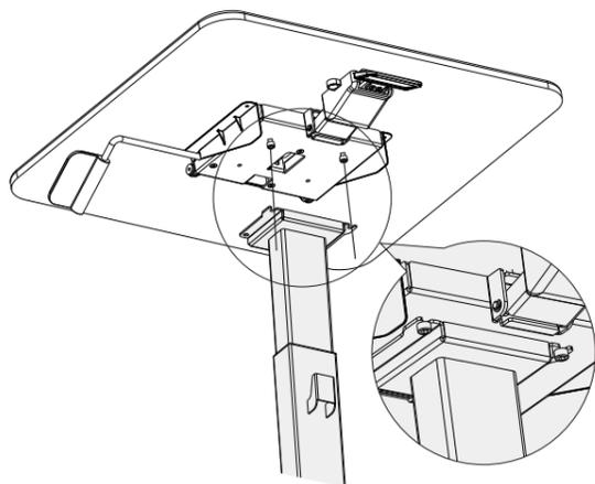
2.4 Screw the other 2 bolts (D2) and tighten all 4 bolts (D2) by using hex key (D3).
