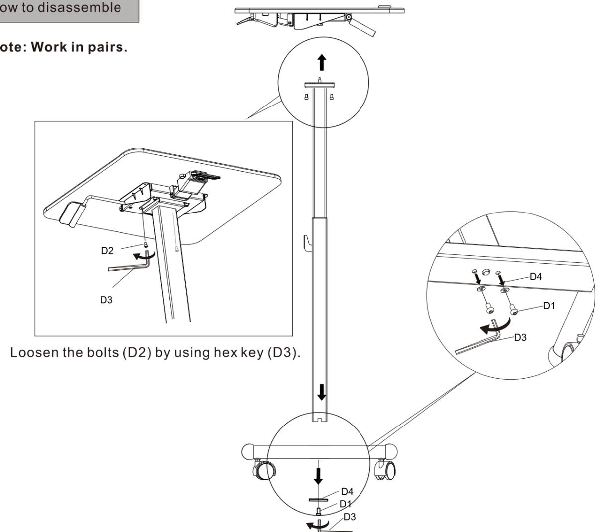
Loosen the bolts (D2) by using hex key (D3).
