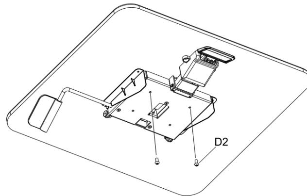
2.3 Attach lifting column (B) to the 2 bolts (D2) under the desktop.
