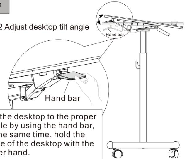
Tilt the desktop to the proper angle by using the hand bar, at the same time, hold the edge of the desktop with the other hand.
