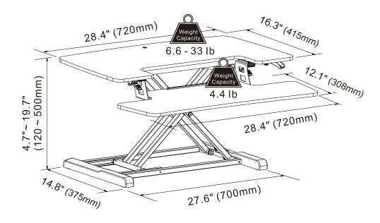
Do not exceed the max. loading capacity as shown.
