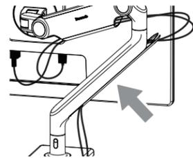
5. Slide the cover down the arm to lock in place, then gently pull the cables through the arm to remove excess slack.
