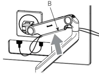
**NOTE:** Leave enough slack in the cables to allow arms to rotate without difficulty.
