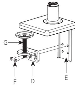
**NOTE:** Clamp Mounts cannot be used to mount the M2.1 to any vertical surface.
