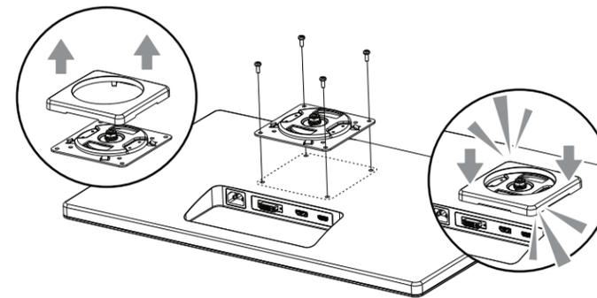
The VESA Bracket features 75mm and 100mm hole patterns. If you need to offset the Bracket from the monitor use the provided Extended VESA screws and Plastic Spacers. You may also use the screws that came with your monitor.
