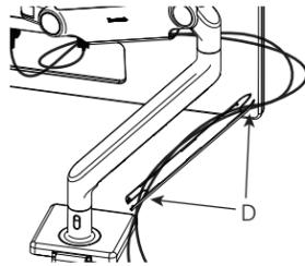
4. Lift the cover and cables up to the lower link, making sure that the cover sits flush with the surface of the arm.
