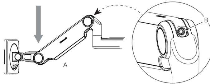
2. Using the 4 mm hex key, turn the Adjustment Screw clockwise (towards **+**) to **increase** force, or counter-clockwise (towards **-**) to **decrease** force. Turn the Adjustment Screw (B) until the monitor is balanced.
