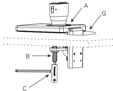
\* If the diameter of the grommet hole is less than 3" (75 mm), a Bolt-Through Mount is required.
