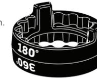
**NOTE:** The stop rings must be configured in such a way that does not allow the monitor to pass behind the rear edge of the unit.
