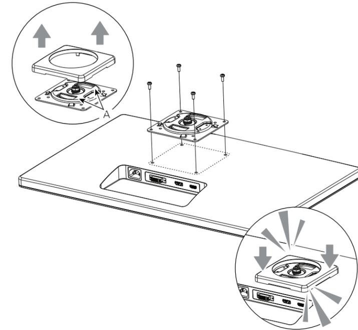
The VESA plate features 75 mm and 100 mm hole patterns. You may also use the screws which came with your monitor to attach the VESA plate. If you must offset the plate from the monitor, use the plastic spacers and extended screws provided.
