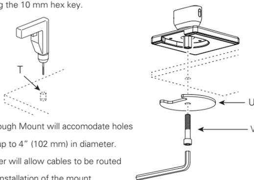
\*\* The Bolt-Through Mount will accommodate holes and grommets up to 4" (102 mm) in diameter. Holes 2" or larger will allow cables to be routed through before installation of the mount.
