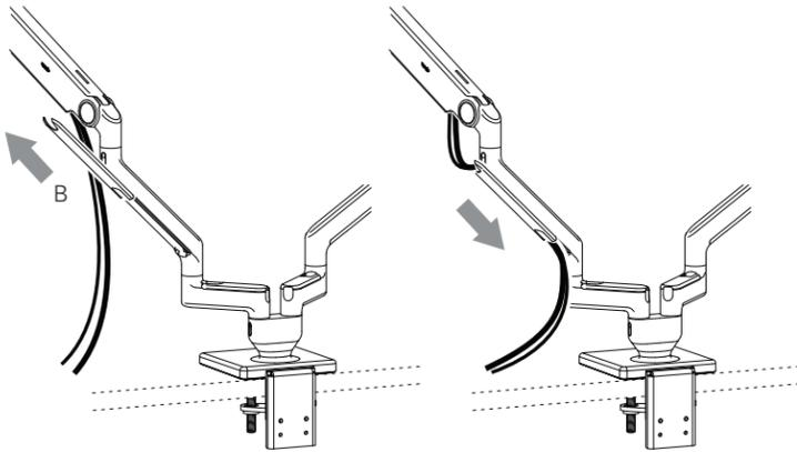
4. Route cables through any remaining links used in your configuration following the same procedure from steps 2-3.
