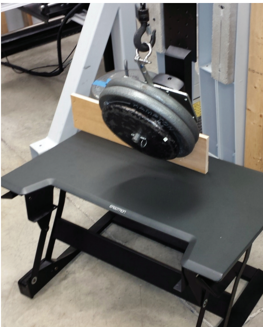
Load testing of tilt mechanism
