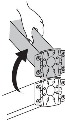
**d3** Re-insert the 4 screws and tighten with the 4mm hex wrench.
