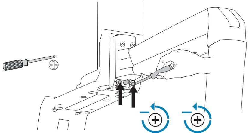
**2** Loosen or tighten this bolt to adjust tilt to desired angle.
