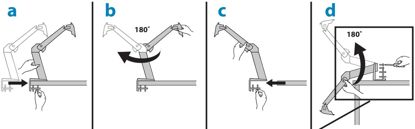
**d1** Remove the 4 screws at the base using the provided 4mm hex wrench.
