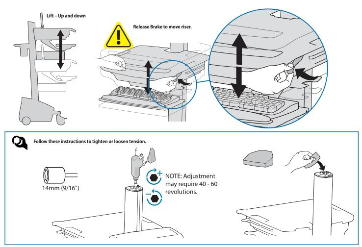
NOTE: Adding more than 3 rows of drawers per cart may mean balanced lift adjustment of the cart may not be possible without reducing weight of LCD, laptop, CPU, and/or drawer contents.
