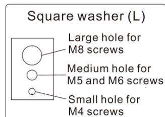
Connect mounting Rails (2) to the back of your TV using four screws (A-I), depending on the size of the VESA holes on the back of your TV and washers (L).
