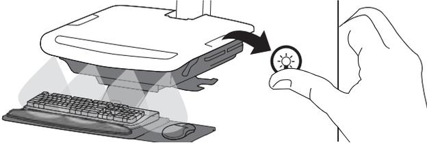
This power system interface will alert you to the percentage of charge remaining in the cart battery with a series of steady or flashing red, yellow or green lights, and an alarm that will beep when charge gets below 10%. Remember, the battery needs to be charged to 100% every day, and you can use the cart while charging, so plug-in cord as often as possible to avoid running out of power!
