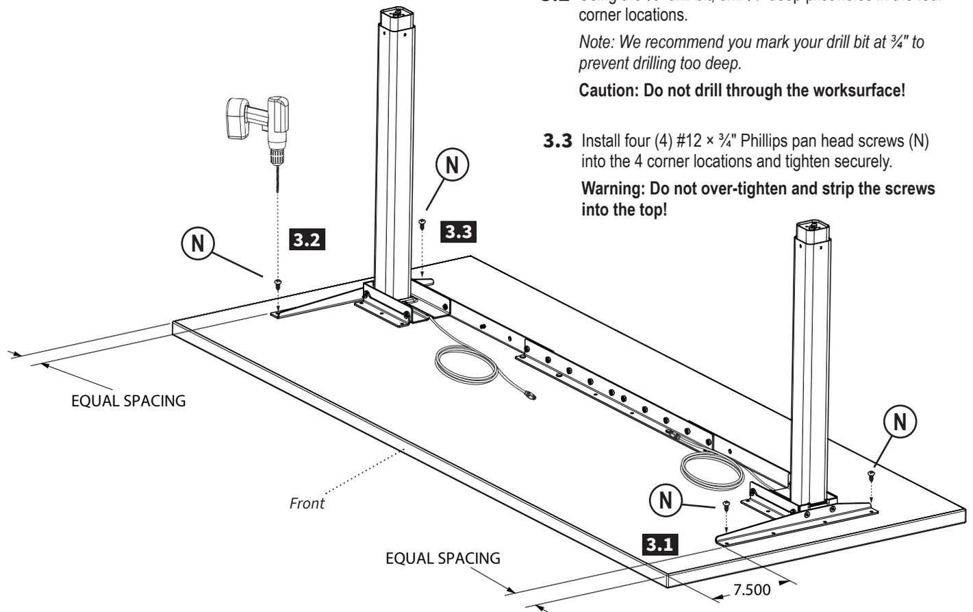
**3.4** Using the  $\frac{1}{8}$ " drill bit, drill  $\frac{3}{4}$ " deep pilot holes in the remaining locations in the brackets on the legs.
