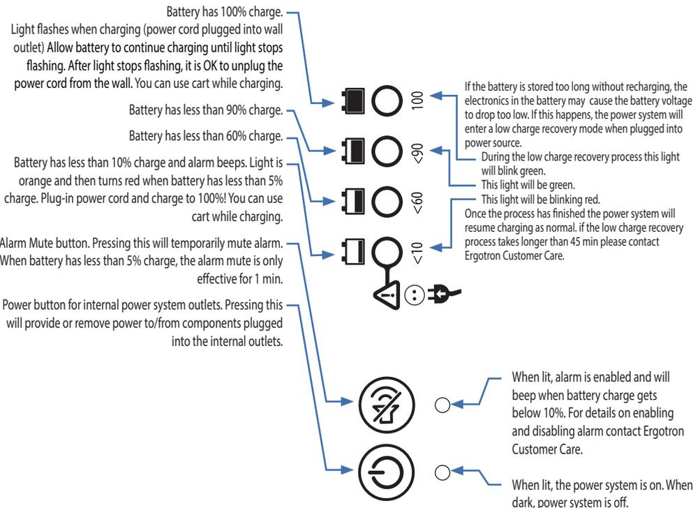
If other lights are flashing red/green it could indicate a power system fault. If this occurs contact Ergotron Customer Care.
