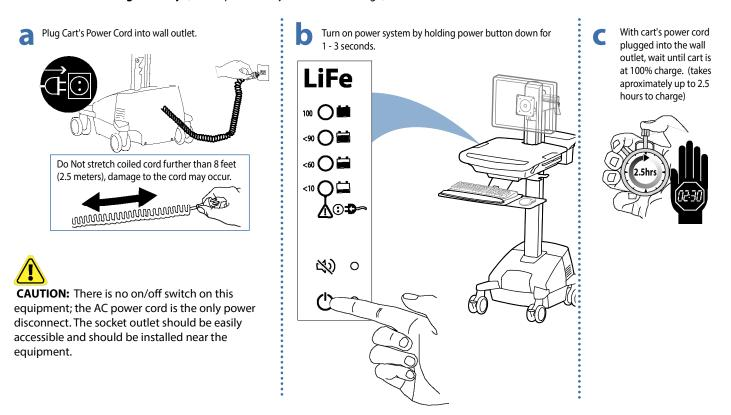
This power system interface will alert you to the percentage of charge remaining in the cart battery with a series of steady or flashing red, yellow or green lights, and an alarm that will beep when charge gets below 10%. Remember, the battery needs to be charged to 100% every day, and you can use the cart while charging, so plug-in cord as often as possible to avoid running out of power!
