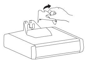
Hang the drawer tabs onto the brackets on the cart.
