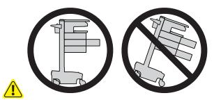
**CAUTION:** Close worksurface before opening drawers. Open only one drawer at a time. Do Not push cart when drawers or worksurface are open. Failure to follow these instructions may cause the cart to be unstable.
