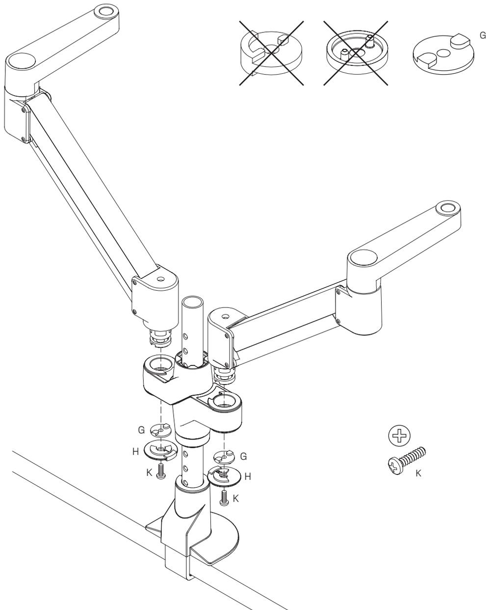
**i** **IMPORTANT:** Install part (H) in the orientation as shown to the left. When washer, part (H), is installed correctly, the arms will not rotate past the back of the mount.
