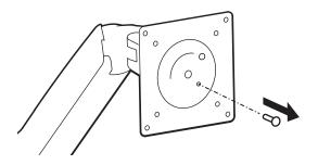
Attach Tablet Mount to 75x75mm or 100x100mm VESA plate.
