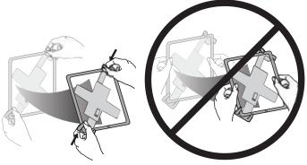
Important! Hold handles when moving mounted tablet around. Not holding handles may cause tablet to come off holder and dropped resulting in possible equipment damage.
