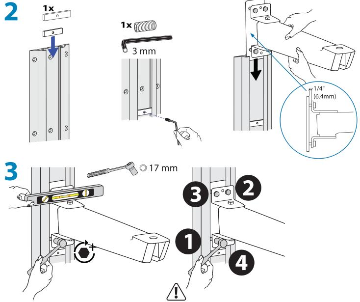
IMPORTANT! Torque bolts in the sequence shown above to a minimum of 50 lb-ft (6.91 kgf-m).
