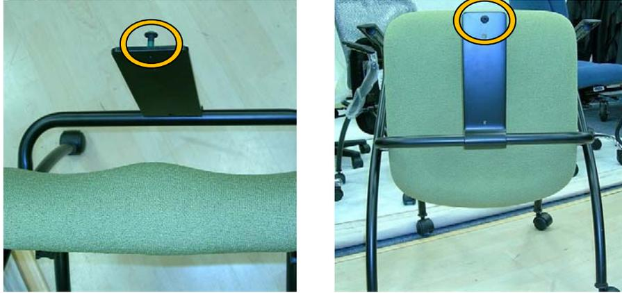
4. Once the Allen Bolt is removed, note the location of the screw hole that it was originally in, and then proceed to the next steps (note that there are **2** holes at the top of the metal upright bar... the one you'll want is the **TOP** hole).
