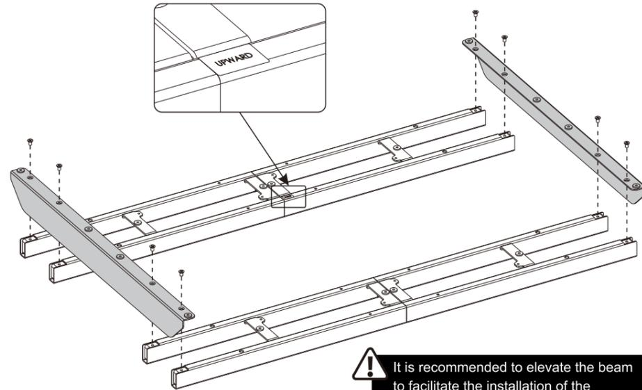
It is recommended to elevate the beam to facilitate the installation of the supporting plate.
