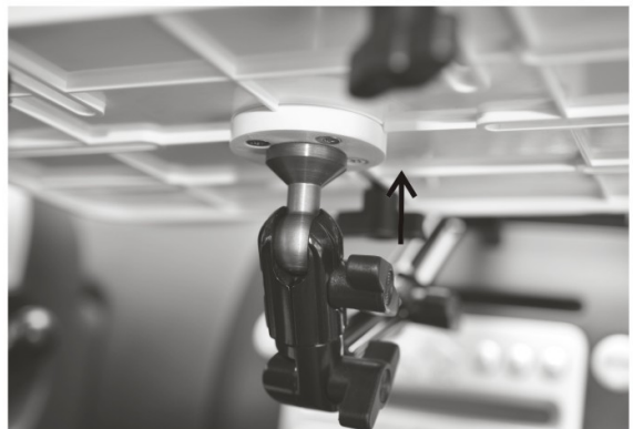
SCREW the TRAY onto the BALL HEAD of the ARM.
