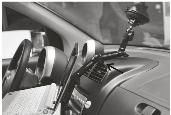
Keep the ARM close to the central console will reduce the vibration.
