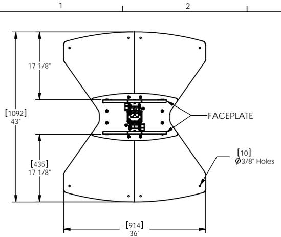
NOTE: CUSTOM INTERAFCE BRACKET NOT SHOWN. THE CUSTOM INTERFACE BRACKET NEEDED FOR YOUR DISPLAY WILL ADD BETWEEN 1/2" AND 2" IN DEPTH AND MAY AFFECT LOCATION OF DISPLAY ON THE MOUNT.
