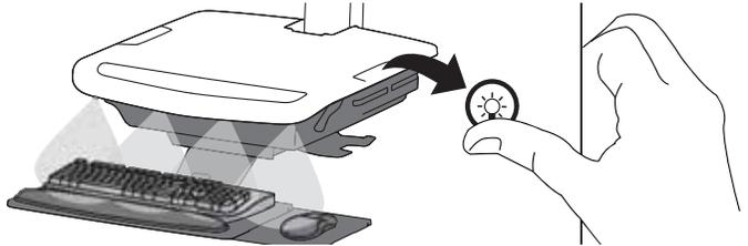
This power system interface will alert you to the percentage of charge remaining in the cart battery with a series of steady or flashing red, yellow or green lights, and an alarm that will beep when charge gets below 30%. Remember, the battery needs to be charged to 100% every day, and you can use the cart while charging, so plug-in cord as often as possible to avoid running out of power!
