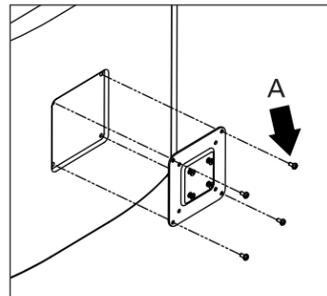
If mounting space for 75mm VESA Bracket is inset into back of monitor, place the four Plastic Spacers (B) between VESA Bracket and monitor (align with hole pattern), and using the Extended VESA Bracket Screws (C), bolt through the Spacers.
