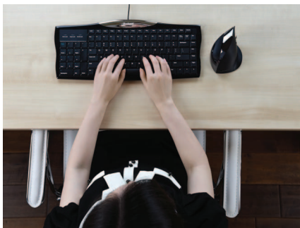
Evoluent's Reduced Reach Right-Hand Keyboard has a number pad on the left side to make space for the mouse.
