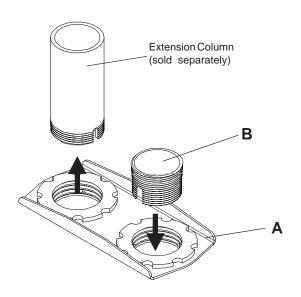
Side to side adjustment is accomplished by rotating adapter bracket (A) about extension column. Lock into position by screwing 1/8" long socket pin screw (C) into hole as shown, jamming screw into threads. For extra security, align one of the three holes in adapter bracket (A) with notch in column, then fasten 3/8" long socket pin screw (D) into hole and through notch.
