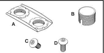
Attach adapter bracket (**A**) to bottom extension column (sold separately). Thread flush mount tube (**B**) into bracket (**A**) as shown until it is threaded all the way down.
