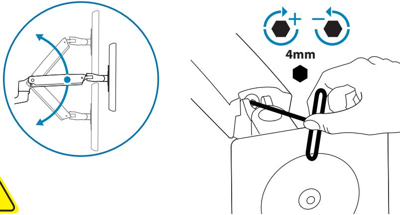
**CAUTION:** DO NOT overtighten fasteners. Overtightening may cause damage to your equipment.
