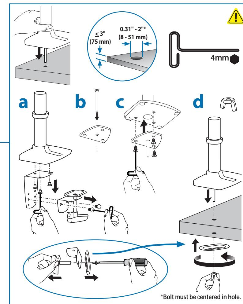
**CAUTION:** For secure arm attachment and to avoid equipment damage, plate must make contact with underside of desk on both sides of the hole.
