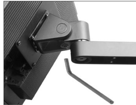
Tilt the monitor so it faces upward and locate the set screw under the tilter. Insert the 7/32" Allen wrench into set screw to adjust the tilt friction.
