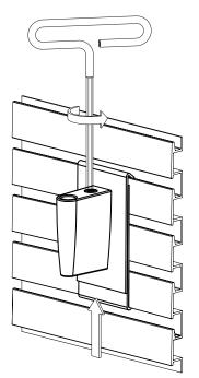
Turn screw counterclockwise to open bracket.Turn screw clockwise to tighten bracket onto slatwall.
