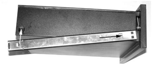
When installing runners on drawer and shelf slide horizontal tab into slot on front of drawer first then push vertical tab up into place. Tab should only slide up into slot on drawer (as shown), if the tab is facing down then the runner is on the wrong side of drawer. Remove and mount on other side.
