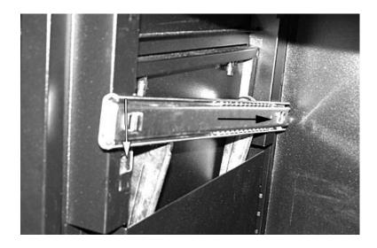
After runners are installed on drawers mount runners on slots inside of unit as shown (note: runners should already be attached to drawer/shelf, the above picture shows runner without drawer for illustrative purposes). Slide horizontal tab into slot at back of unit first, then push vertical tab down into slot at front of unit. If vertical tab is facing up the runners are on the wrong side of the drawer. Remove and mount using above instructions.
