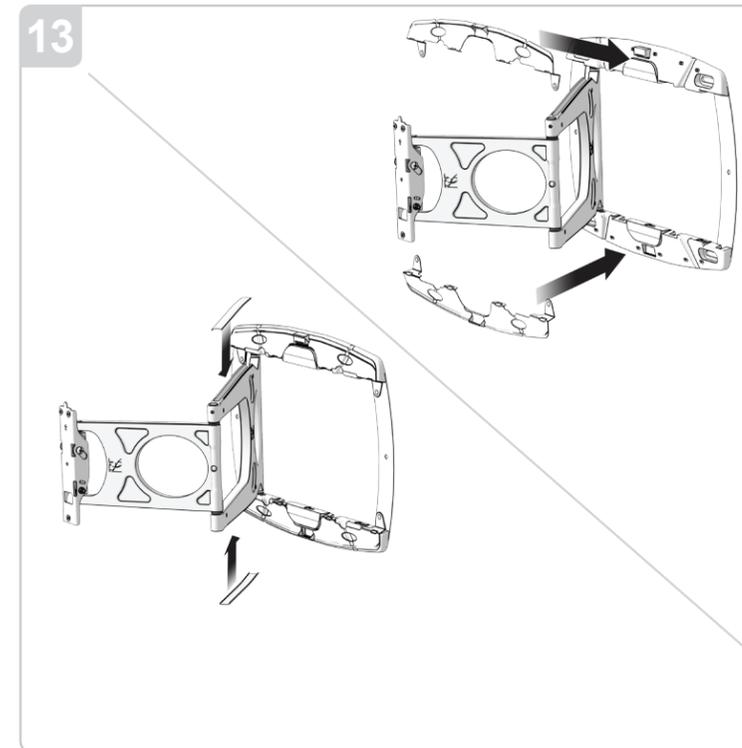
Install the upper and lower "push on" plastic "beauty covers" to the upper and lower wall plates. Reinstall the upper and lower plastic cable covers to the mounts main swing arm.
