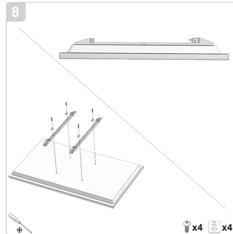
Place the display face down on a smooth flat surface. Place the left and right mounting brackets over the four mounting points on the rear of the display arrow pointing up to the top of the display, making sure the brackets are lined up with the center top to bottom on the display.
