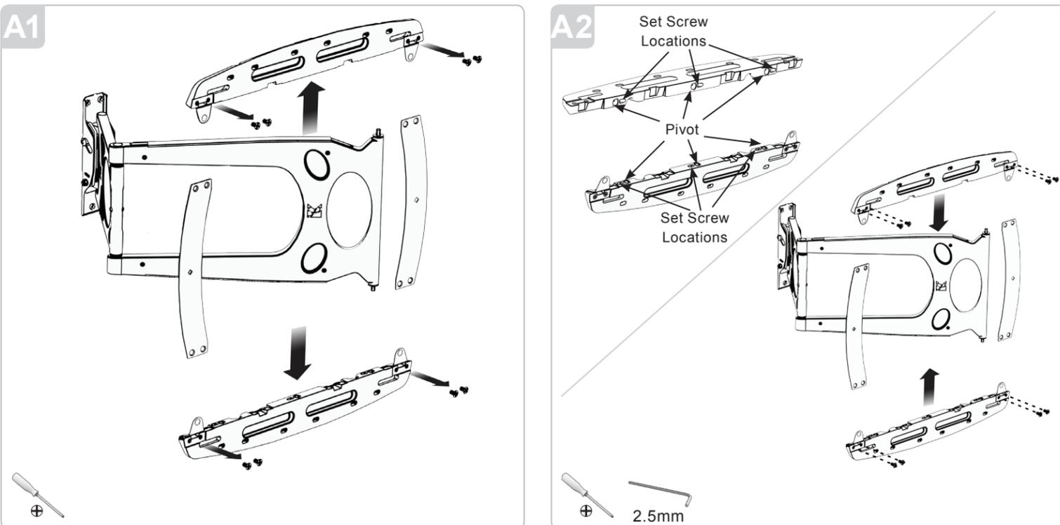
Remove the plastic hole covers from the upper and lower plates. Loosen the (2) set screws on the plate using the 2.5mm allen key supplied. Reposition the upper and lower pivot rods to mate to either the center or right side pivot receiver holes, push the upper and lower plate fully on to the rods, and re-tighten the set screws. Reinstall the side plate with the eight flat head screws and confirm they are secure. Reinstall the round plastic hole covers.
