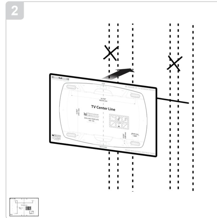
Take the thick cardboard mounting template supplied and place it over the mounting studs with the screen center facing up. Confirm that the template is level horizontally and that the wall place outline is to the center of your desired height.
