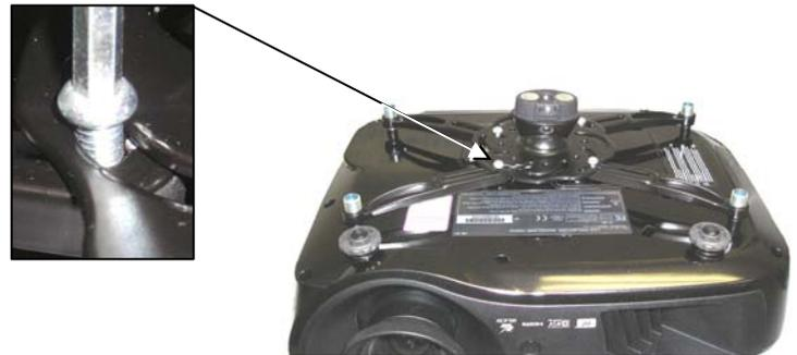
4. Align the projector plate to the mounting legs.
