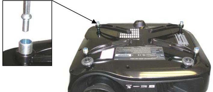
1. Locate the mounting points on the bottom of the projector (see arrows above for mounting point recognition).
