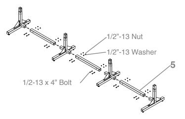
Using 1/2"-13 bolt, nut and washer, attach part# 5 (8900-007-101-XX) to the previously assembled components. The MVW-3X3-55 has three of part# 5 and the MVWS-2X2-4655 has two of part# 5.
