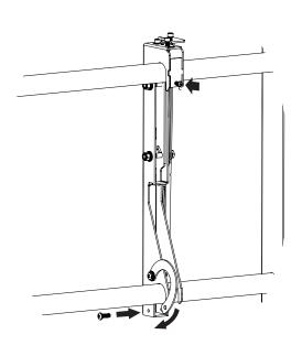
After the display is on the stand in the proper position, tighten the back safety screw so that it is snug (DO NOT OVER TIGHTEN). Rotate the bottom mount safety latch around the vertical mounting bar, and secure it with the previously removed screw.
