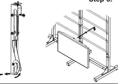
For each display on both of the brackets, back out the rear safety screw to clear the horizontal mounting bar. Remove the screw securing the bottom hook and spin the hook up so that it will clear the horizontal mounting bar. The display can now be installed onto the horizontal tubing.
