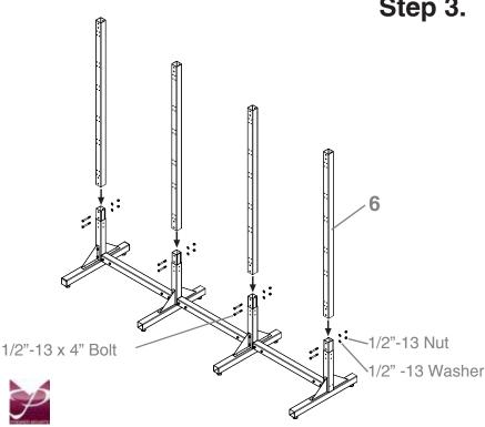
Using 1/2"-13 bolt, nut and washer, attach part# 6 (8900-007-111-XX for MVWS-3X3-55, 8900-006-111-XX for MVWS-2X2-4655) to the assembly. The MVW-3X3-55 has four of part# 6 and the MVWS-2X2-4655 has three of part# 6.
