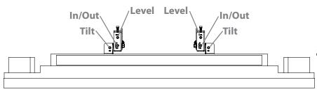
Each bracket has fine tune adjustments that can adjust the level, tilt and in/out of each individual display. Be careful NOT TO OVERTIGHTEN these adjustment screws.
