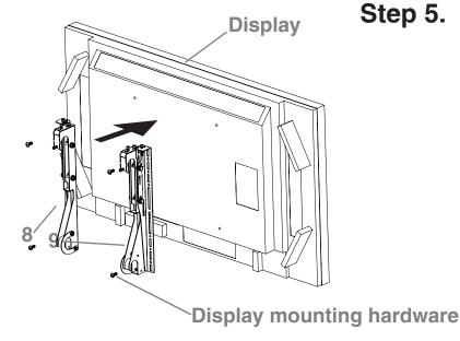
Attach part# 8 (8900-007-170-XX) and part# 9 (8900-007-160-XX) to each display using the correct size hardware for the display used. Use the vesa mounting holes pointed out in the picture.
