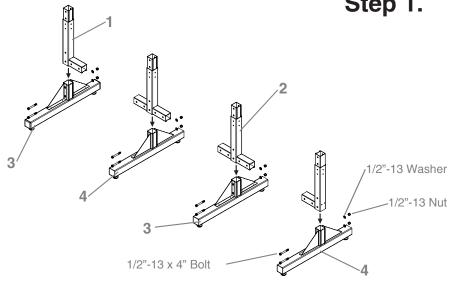
Using 1/2"-13 bolt, nut and washer, bolt together part# 1 (8900-007-180-XX) and part# 2 (8900-007-190-XX) to part# 3 (8900-007-110-XX) and part# 4 (8900-007-120-XX). The MVWS-3X3-55 has four sections and the MVWS-2X2-4655 has three sections.
