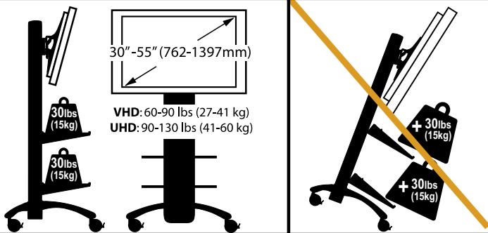
DO NOT load the Cart / Stand past maximum weight capacity. DO NOT mount a display larger than the recommended size. Failure to comply with warning may result in Cart / Stand instability leading to equipment damage or personal injury.
