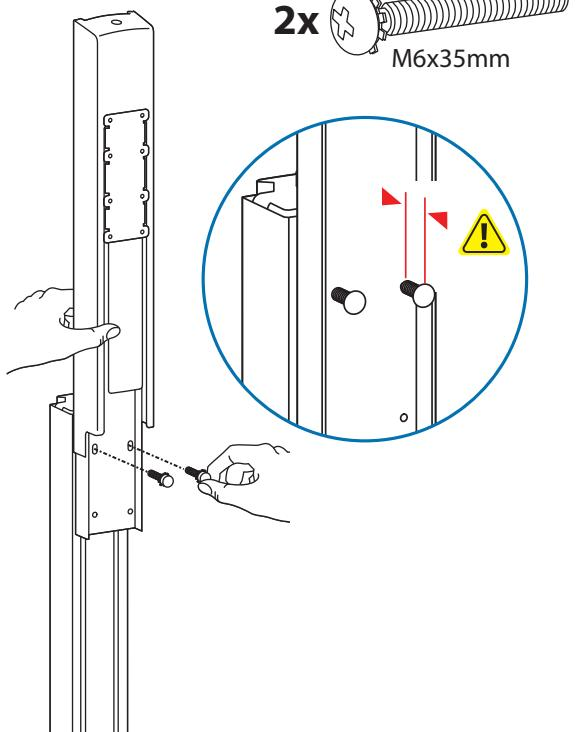
**WARNING:** Stored Energy Hazard: The lift mechanism in the tower is under tension and will move up rapidly, on its own, as soon as attached equipment is removed. For this reason, DO NOT remove equipment or make adjustments to lift tension unless the front assembly has been moved to the highest position on the tower! Failure to follow this instruction may result in serious personal injury and/or equipment damage!
