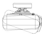
YAW 360° (when attached to an extension column), +/- 15° (when flush mounted)
