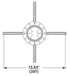
\*Mounting holes on projector must be within a 15.63 in diameter in order to use this product.
