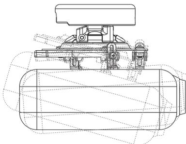
YAW 360° (when attached to an extension column), ±30° (when flush mounted)
