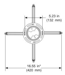
\*Mounting holes on projector must be within a 16.6" diameter in order to use this product.
